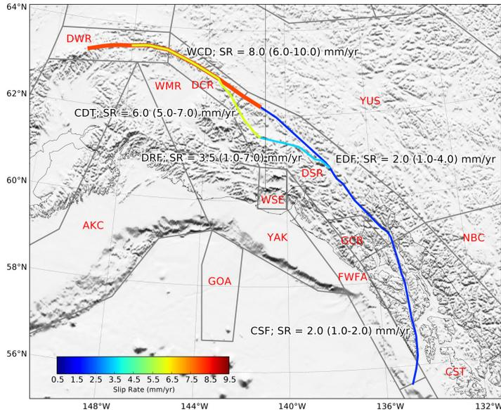
**Figure 4 – Surface projection of crustal fault sources in Yukon and Alaska coloured by slip rate. Published slip rates are used to estimate the seismic moment rate and develop magnitude-frequency distributions. WCD = Western-Central Denali fault; CDT = Central Denali-Totshunda faults; EDF = Eastern Denali fault, and; DRF = Duke River fault.**
