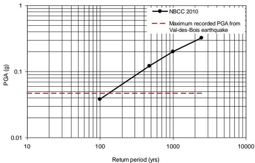
Figure 6: Hazard curve for PGA on Site Class C in Ottawa, showing that the Val-des-Bois earthquake shaking represents about the 1/150 year shaking level.
