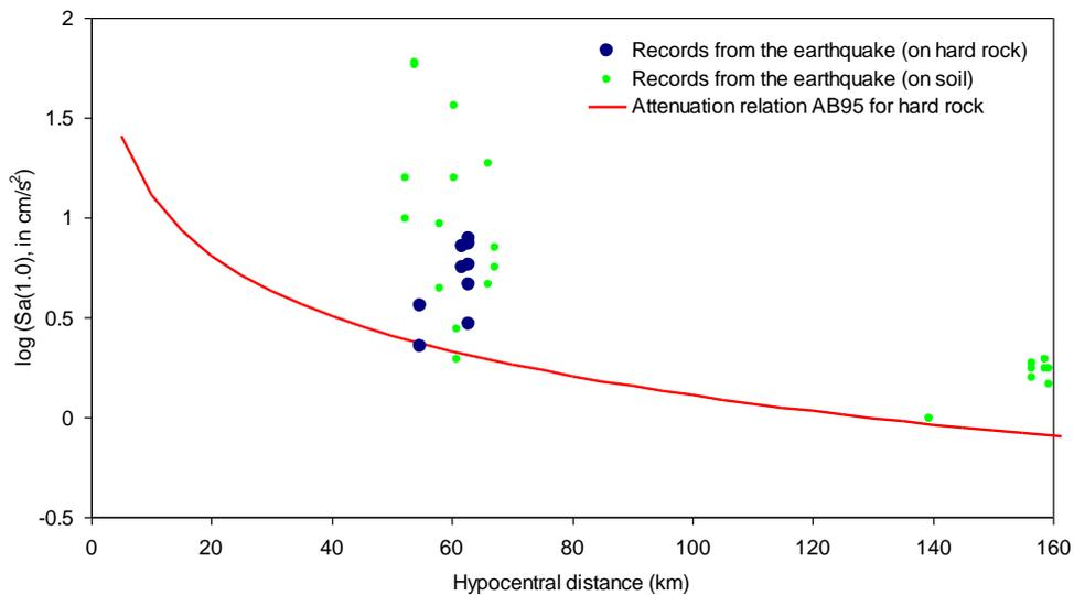
Figure 4: Attenuation relation for  $Sa(1.0)$  for hard rock (NEHRP soil class A) used for Eastern Canada together with  $Sa(1.0)$  values for horizontal components recorded at hard rock and soil sites.
