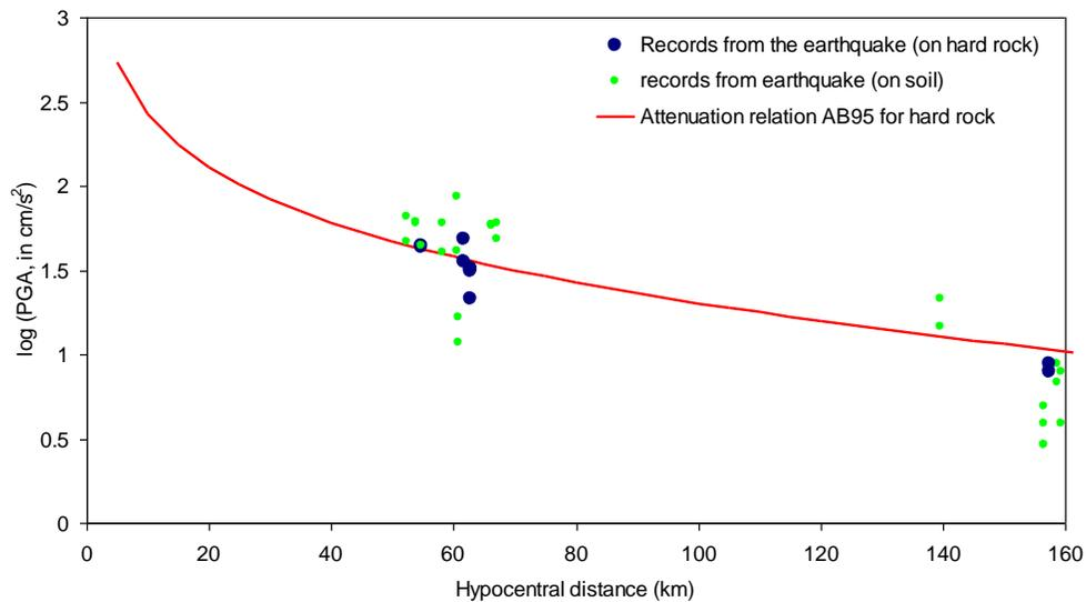
Figure 2: Attenuation relation for PGA for hard rock (NEHRP soil class A) used for Eastern Canada together with PGA values of horizontal components recorded at hard rock and soil sites.
