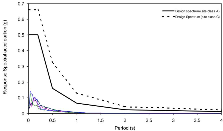
Figure 5: Comparison of the response spectra for records obtained at hard rock sites in Ottawa with the NBCC2010 design spectra for Site Class A and C.
