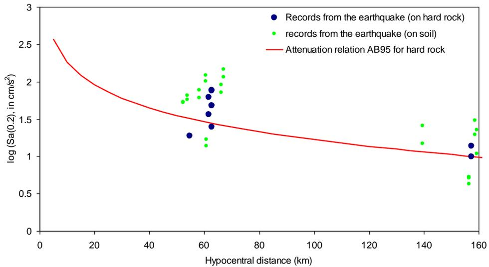
Figure 3: Attenuation relation for  $Sa(0.2)$  for hard rock (NEHRP soil class A) used for Eastern Canada together with  $Sa(0.2)$  values for horizontal components recorded at hard rock and soil sites.
