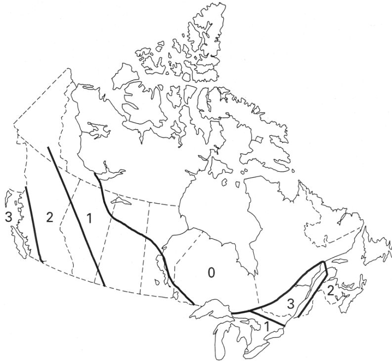
Fig. 2. Seismic zoning map from the 1953 National building code of Canada (NRCC 1953).
