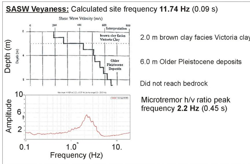
Figure 4. Comparison of peak frequency at SASW Veyaness located atop of a glacial drumlinoid ridge of dense glacial Pleistocene material (till) from SASW testing and microtremor recording.
