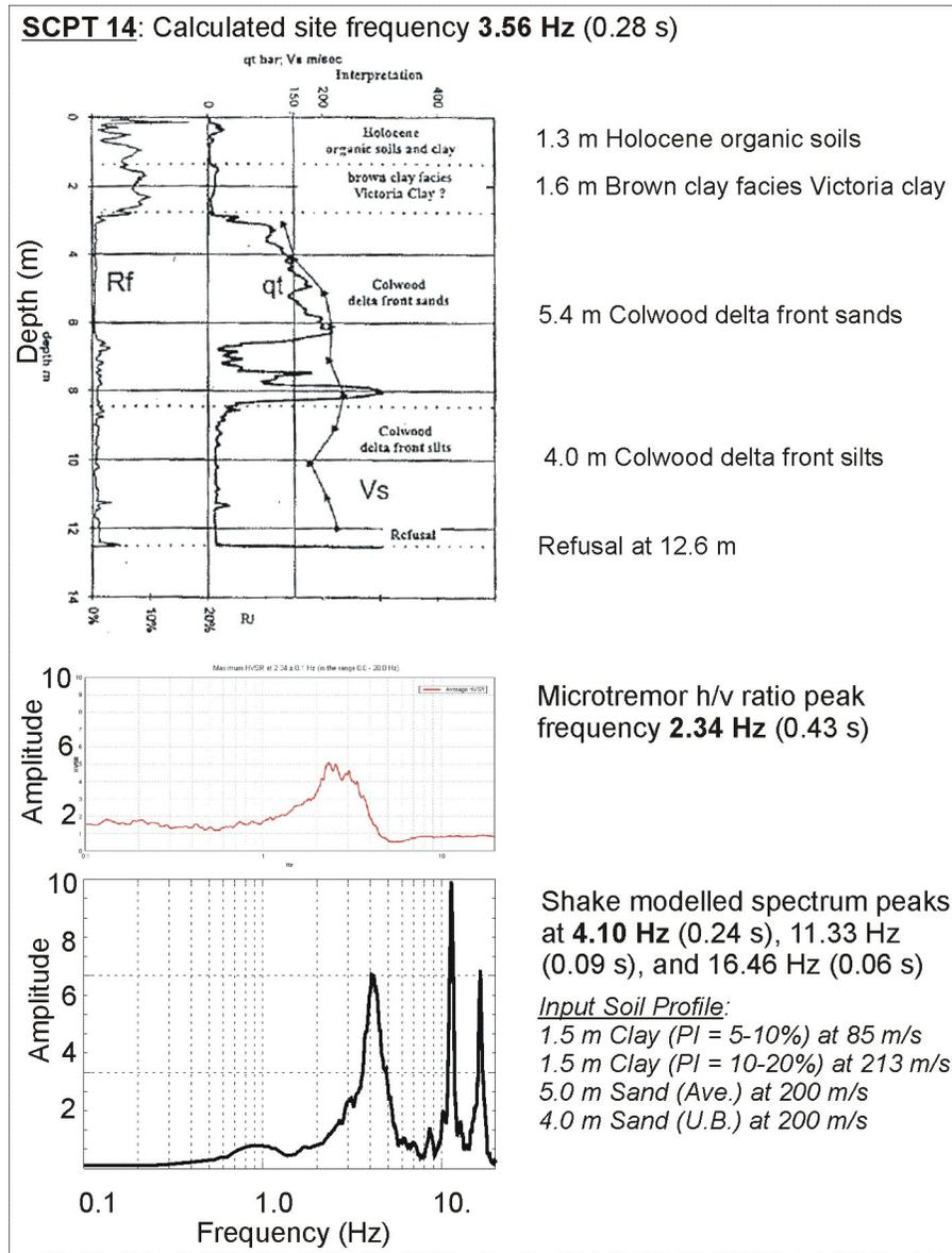
Figure 2. Comparison of peak frequency at SCPT 14 located on the Colwood sand and gravel delta front from SCPT measurements, microtremor, and SHAKE modelling. SCPT parameters:  $V_S$  = shear-wave velocity, qt = tip resistance, and Rf = friction ratio.
