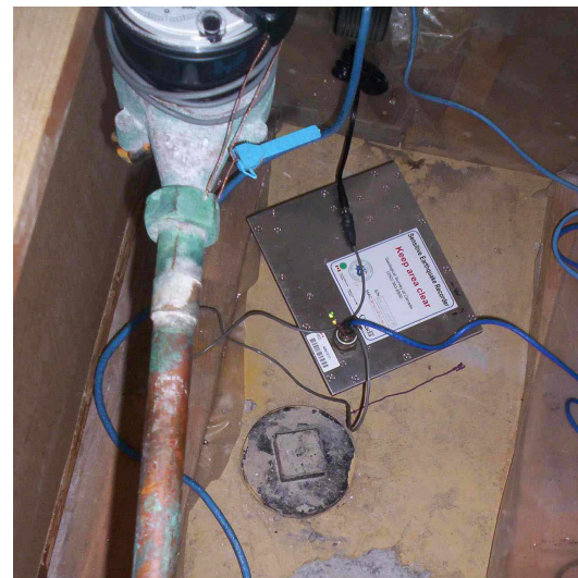
Figure 2. Site OT002. (Above) View of basement under construction in 1986. The IA is now installed under the red arrow. Current house is similar to the ones in the background. (Right) The IA is oriented and then bolted to the floor slab.
