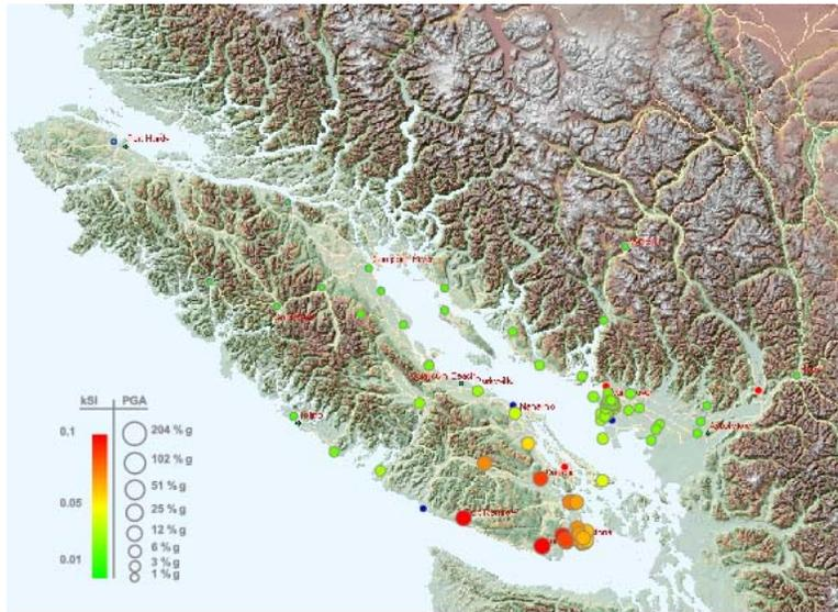
Figure 2. Spectral intensity measured at the instrument location is color-coded, PGA varies with symbol size.
