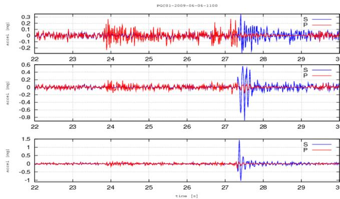
Figure 1. Discriminating P- (red) and S-Phases (blue) for separate detection.
