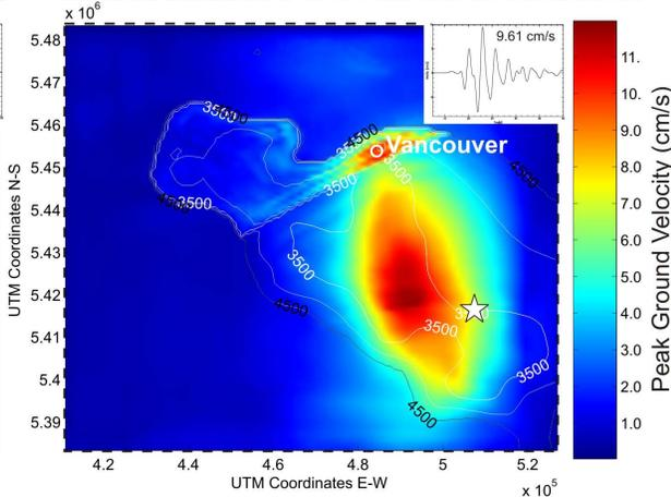
Figure 3. Peak ground velocity (EW motion) maps of the Georgia basin region from simulation of a  $M_w$  6.8 in-slab event at four different positions (white stars) within the 3D model overlaid with velocity contours of the 3D model at 750-1000 m depth as in Fig. 1. Synthetic waveforms in upper right of each map represent simulated ground motion in Vancouver (open white circle). The largest ground motion simulated in Vancouver (9.6 cm/s) occurs when the source is located to the SE (location #4).
